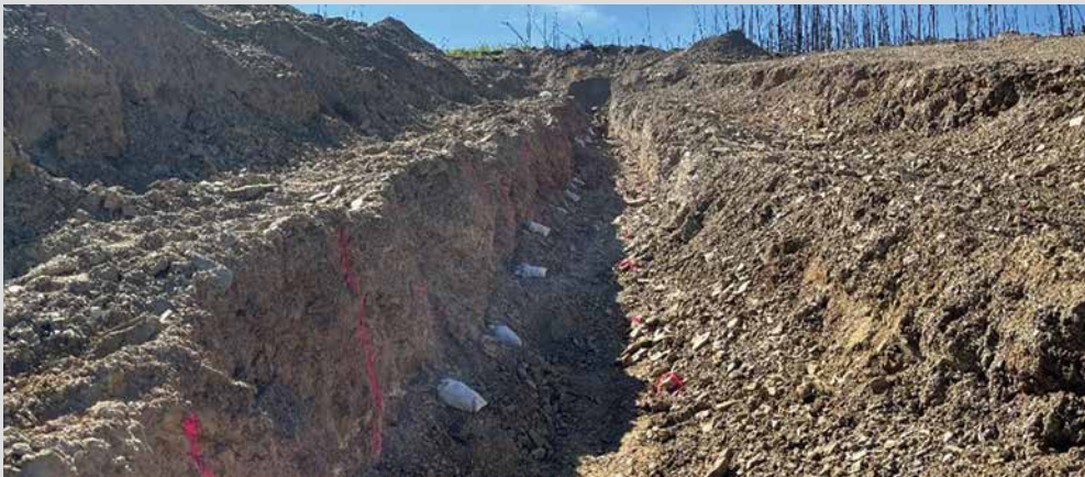
Notice the white sample bags and even spacing? After the geologist takes their samples, the trench is filled back in and vegetation is placed back on top.
