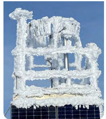
Iced weather monitoring station
